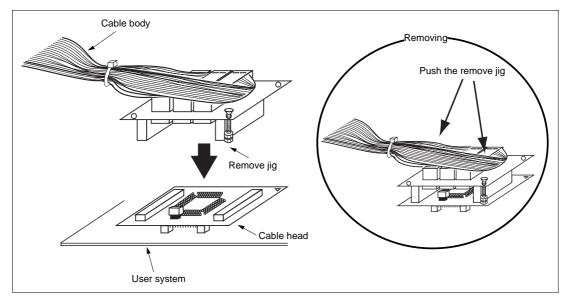
Figure 5 Fastening Cable Body
